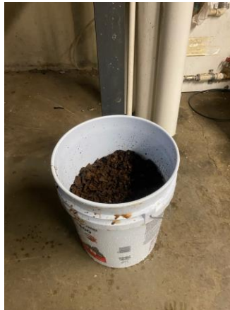
Scale collected from old condensate pipes
